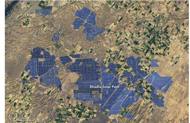
The Bhadla Solar Park (Rajasthan), the worlds largest, spreads over 56 km 2 with a capacity of 2.2 GW
